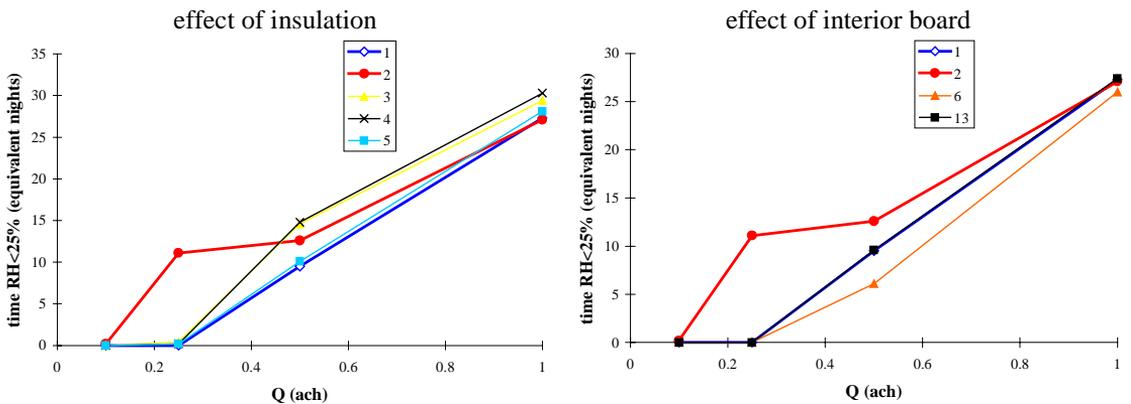
Figure 84. Time that the indoor humidity is less than 25% RH during occupation as a function of the outdoor ventilation rate (Belgium).
