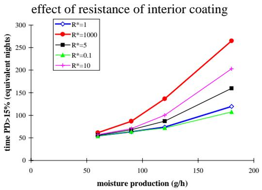
Figure 98. Time that the percent dissatisfied with warm respiratory comfort is greater than 15% during occupation as a function of the moisture production rate (Belgium).
