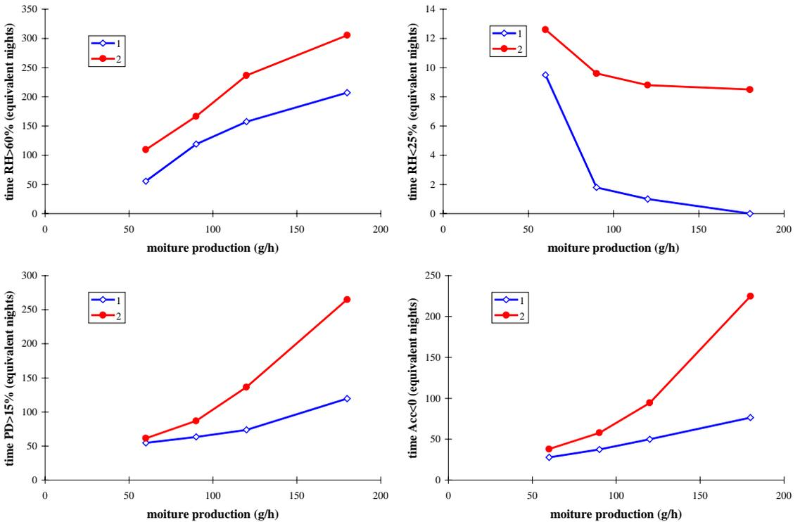
Figure 95. Time that the indoor conditions are outside certain limits during occupation as a function of the moisture production rate (Belgium).
