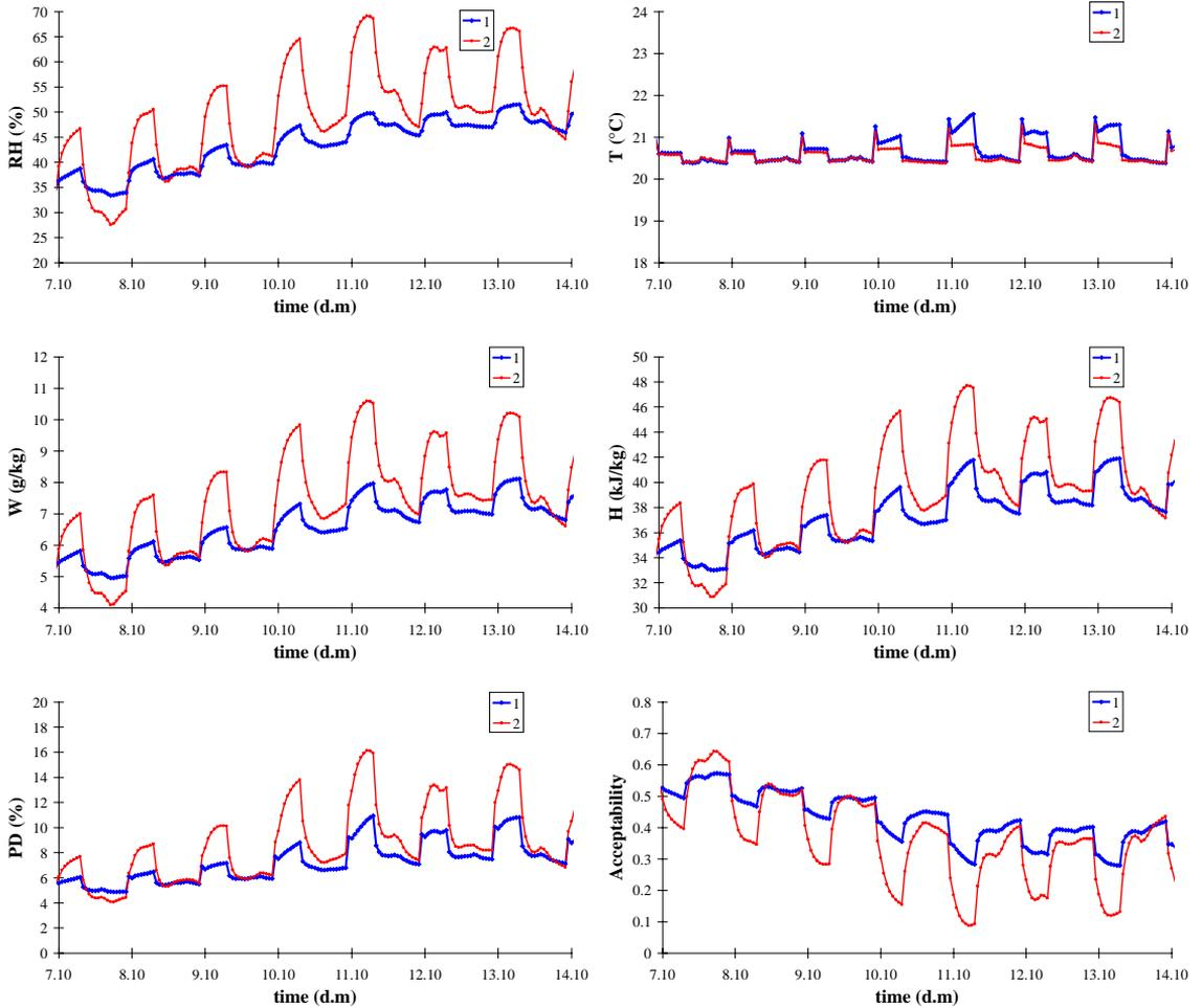
Figure B.10. Temporal variation of the important indoor air variables during a period of increasing outdoor humidity in October in Finland.
