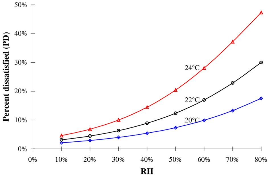
Figure 4. Percent dissatisfied with warm respiratory comfort at various temperatures and relative humidities.
