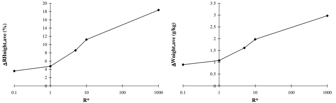
Figure 66. Average increase in relative and absolute humidity during the night as a function of the vapour resistance ratio.
