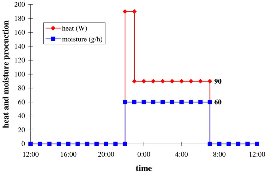
Figure 8. Heat and moisture production in the bedroom.
