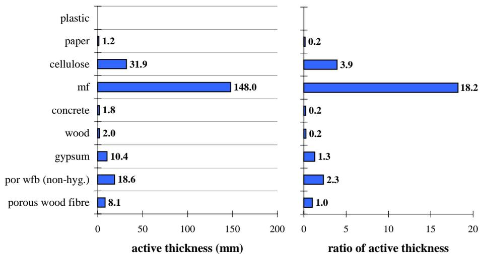
*Figure 16. Estimated active thickness for the materials used in this report and the ratio of the active thickness to the active thickness of porous wood fibre board. The active thickness represents the distance at which the variation of RH in the material is about one third of the variation in the room during a 24 hour cycle. The active thickness will approximately double if a criterion of 10% is used.*
