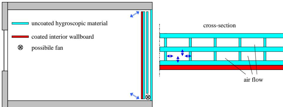
*Figure 114. A possible small but highly active moisture storage device.*
