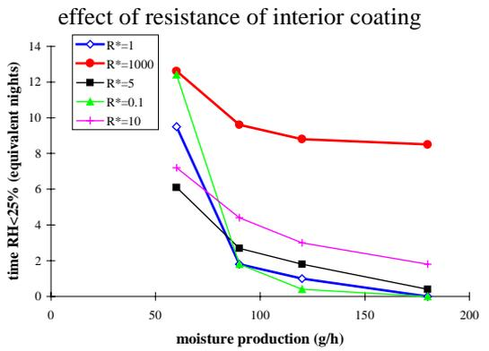
Figure 97. Time that the indoor humidity is less than 25% RH during occupation as a function of the moisture production rate (Belgium).
